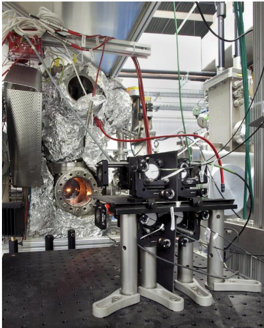
Picture 2: Exterior view of the experimental setup. Gas-cell setup used at GSI/FAIR for the investigation of the short-lived fermium isotopes with the glowing desorption filament.
