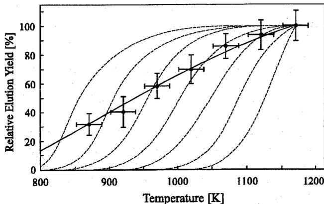
Fig. 1: Relative elution yield of <sup>169</sup>W as a function of the column temperature in isothermal on-line gas chromatography: experimental data and calculated yield curves
