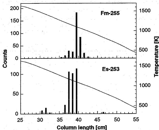
Fig. 1: Thermochromatogram of  $^{253}\text{Es}$  and  $^{255}\text{Fm}$  on a V column
