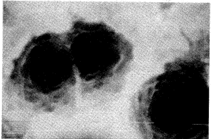
Fig. 2. Surface pores of about 2 \mu\text{m} diameter and depth (scale bar: 1 \mu\text{m} )
