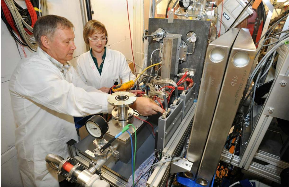
Dr. Alexander Yakushev, spokesperson of the experiment, and Dr. Lotte Lens are fine-tuning the data acquisition system for the registration of flerovium atoms. The vacuum chamber containing the COMPACT chromatography channel can be seen in front; in the background, the last red magnet from the TASCA separator is visible. (Photo: G. Otto, GSI).
