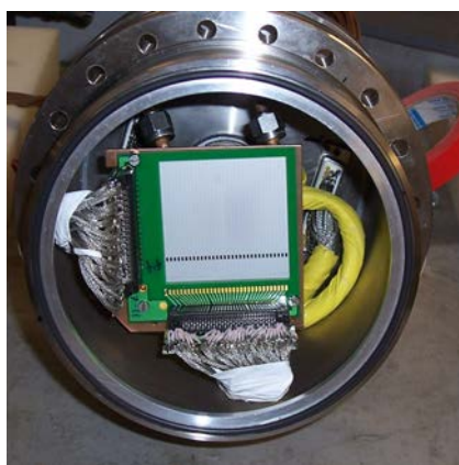
Figure 62: Photograph of the DSSSD inside the detector chamber, which was installed behind TASCA.
