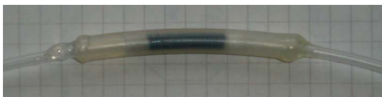
Figure 35: Photo of a charcoal trap. Picture taken from [118]
