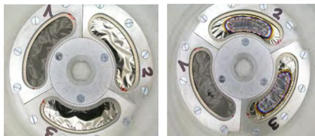
Figure 1: Target TN8 before (left) and after irradiation (right) with a <sup>40</sup>Ar-beam of 1 µA<sub>part</sub> maximum intensity.
