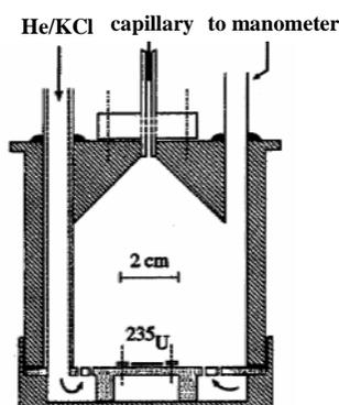
Fig.1: Set-up of the  $^{235}\text{U}$ -target and recoil chamber used for fission product production
