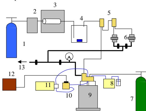
**Fig.1:** Experimental set-up. 1 Helium, 2 mass-flow-controller, 3 KCl cluster oven, 4  $^{227}\text{Ac}$  emanating source, 5 gas-jet switches, 6 direct catch and waste unit, 7 Nitrogen, 8 Acetone pump, 9 ALOHA, 10 electrodeposition cell, 11 electrolyte pump, 12 potentiostat, 13 to the ventilation system. Gas jet flow: black line, vacuum system: thick black line, liquid flow: blue line
