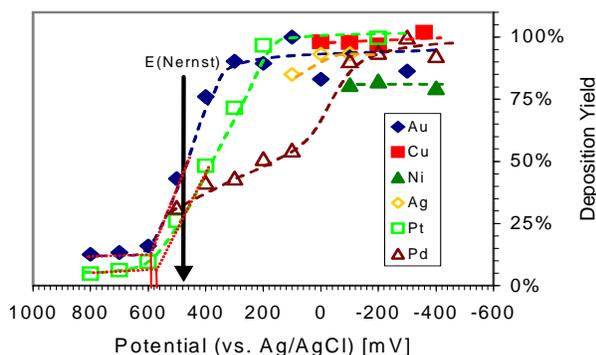
**Fig.1:** Electrodeposition yield vs. electrode potential for the deposition of  $^{197g}\text{Hg}$  on various metal electrodes. In the experiments with Ag, Au, and Cu, 0.1M  $\text{HNO}_3$  and with Pt, Pd, and Ni, 0.1M  $\text{HCl}$  was used as electrolyte
