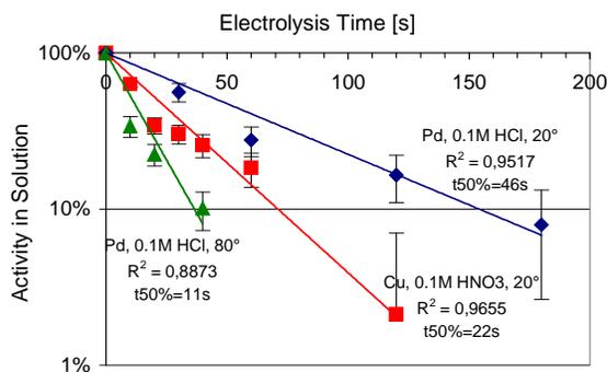
**Fig.2:** Electrodeposition speed vs. electrolysis time for the deposition of  $^{197g}\text{Hg}$  on Pd and Cu. Electrolytic systems: Pd / 0.1M  $\text{HCl}$  / 20° / -500mV; Cu / 0.1M  $\text{HNO}_3$  / 20° / -300mV; Pd / 0.1M  $\text{HCl}$  / 80° / -500mV
