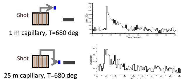
Figure 1: 511 keV gamma emission following the  $\beta^+$  decay of  $^{63}\text{Zn}$  after gas collection utilizing a 1 m (top) and 25 m (bottom) capillary transport line; the decay of the 511 keV gamma line confirms the 38 sec half-life of the  $^{63}\text{Zn}$  isotope.
