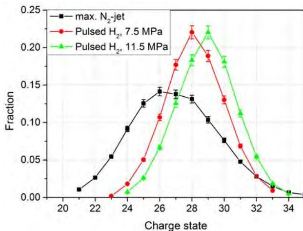
Figure 1: Comparison of the charge state distributions of <sup>238</sup>U ions after passing through the charge stripper applying different gas targets and back-pressures on the gas inlet.
