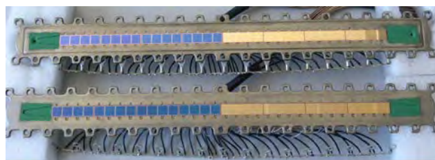
Fig. 1: COMPACT detector array with SiO 2 and Au surfaces.
