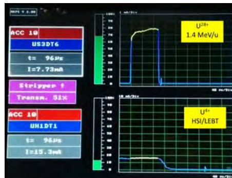
Fig. 2: Beam transformer measurement after careful optimization of a VARIS-uranium beam.
