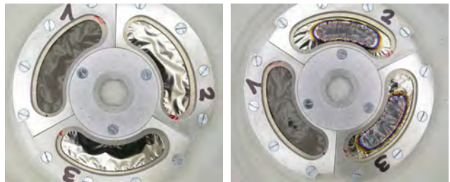
Figure 1: Target TN8 before (left) and after irradiation (right) with a 40 Ar 10+ -beam of 1 µA part maximum intensity.
