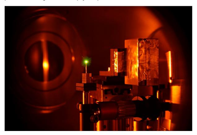
A material sample is placed in the target chamber of GSI's high-performance laser PHELIX. With the aid of the high-intensity laser beam protons are then accelerated out of its back-surface. Photo: V. Bagnoud, Edit: P. Boller / GSI
